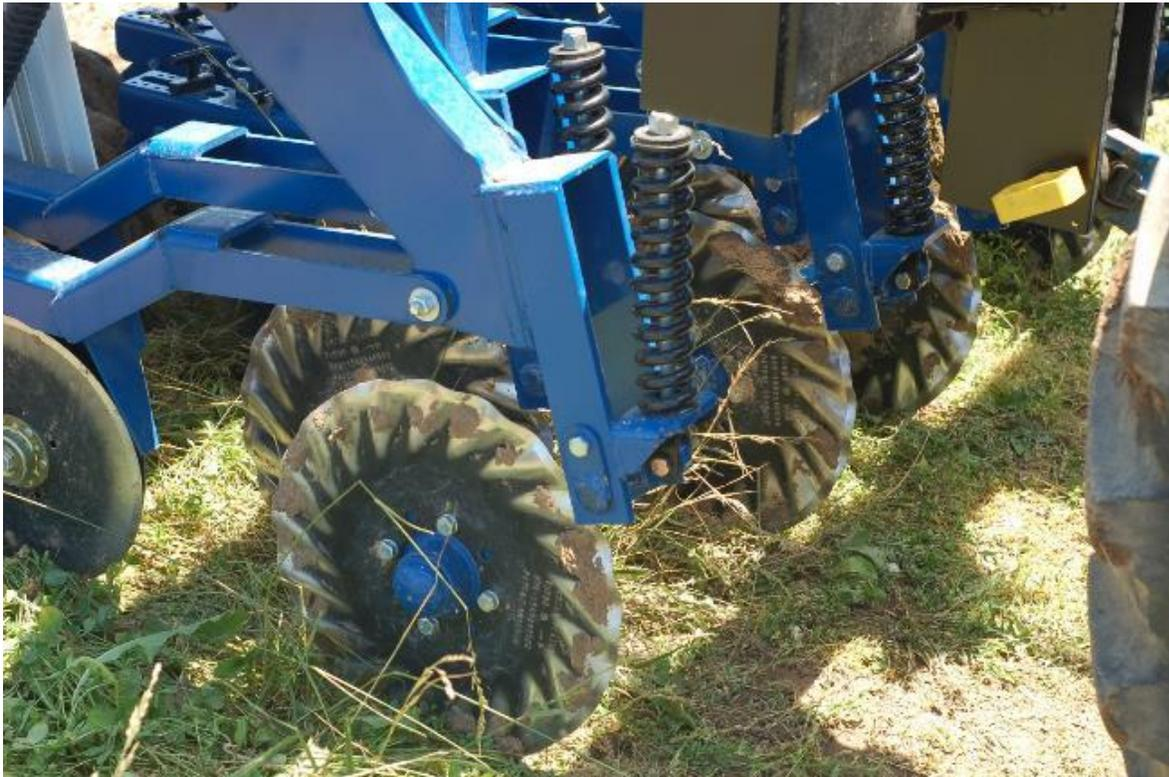
Coulters and disk openers on interseeder
