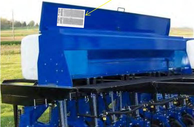
High and low range gears are interchangeable, look for the door sticker to indicate which range
