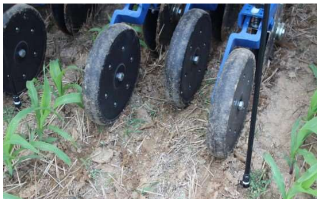
Closing wheels and N application tube - latest design components of Interseeder
